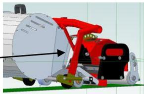
13. The GT190 Fraise-Groomer works different compared to any other verticutter or groomer. Thanks to the integrated gearbox, the rotation direction of the blades will be reversed. This means that the blades of the GT190 rotate against driving direction. This rotation direction helps the blades to `lift-out` the material instead of dragging it through the slit.
